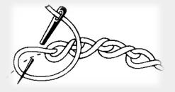
Unlike chain stitching which loops 1 thread over & over and can lead to continuous rips, lock stitching twists 2 threads and locks each stitch to prevent rips from running.
